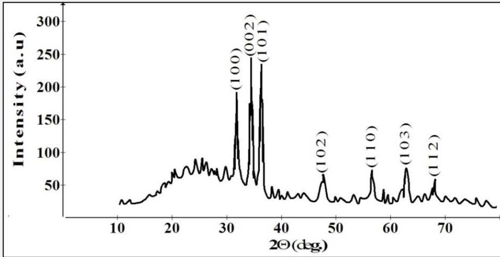
Figure 1. XRD of Zn oxide nanoparticles film on a glass substrate.
