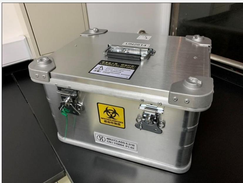
**Figure 2.** The UN2814 specimen transport box.
