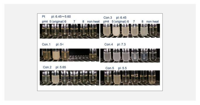
Figure 1. Heat coagulation test under various pH.
